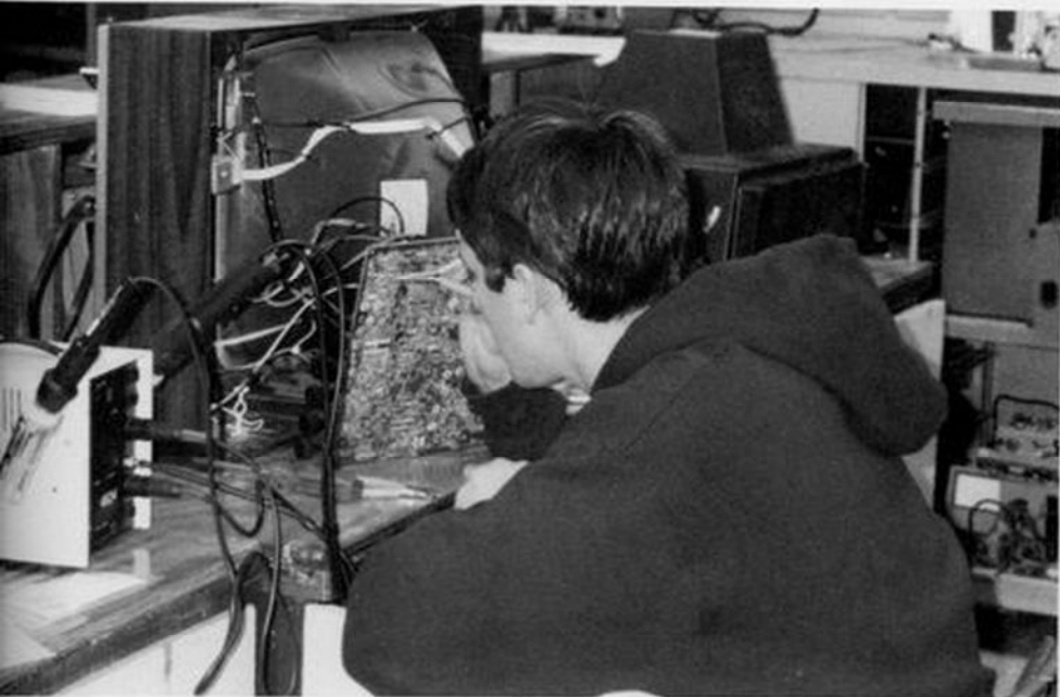
Senior Jonah Bauserman is repairing a T.V. by replacing an integrated circuit.
